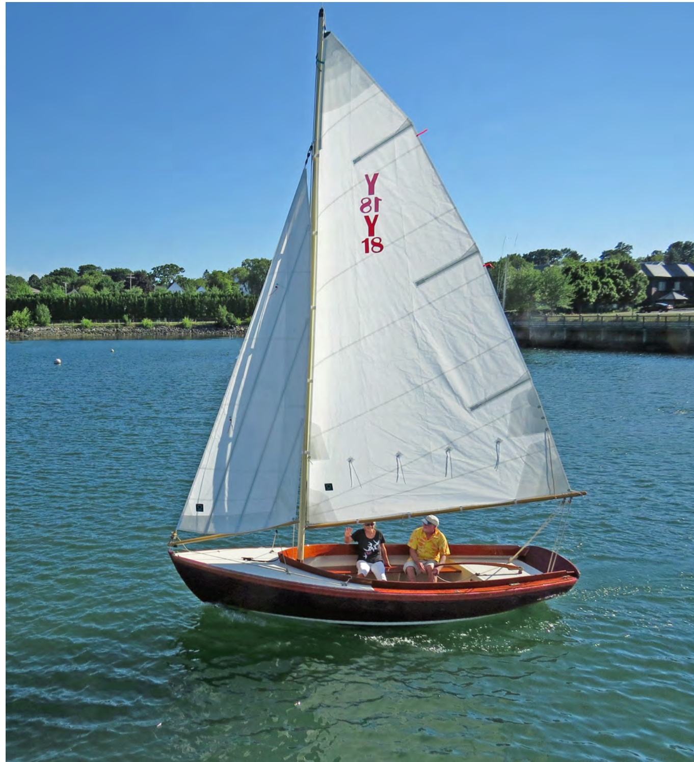
The primary difference with its predecessors is the spade rudder. The vertical battens in the jib prevent it "kiting" and twisting off, increasing her speed significantly.
