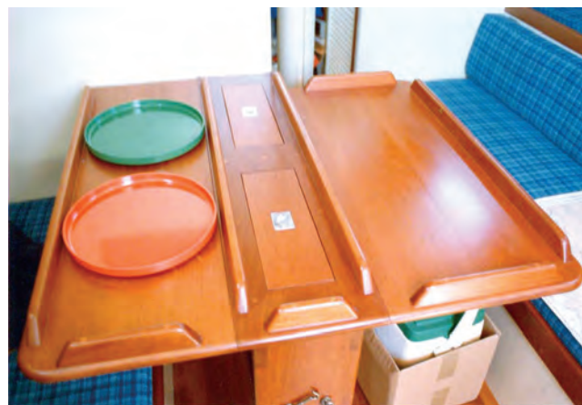
The table was sized to the plates, which just fit between the fiddles. Even the plates had "fiddles!"
