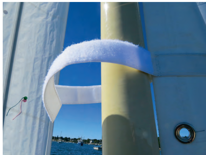
Strap open. The simple Velcro-strap attachments render tracks and slides, and mast hoops obsolete.
