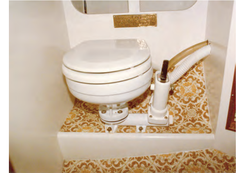
The head sat on a flat plinth that was just big enough for it to fit. Quite a bit of the slant of the hull was there both in front of the plinth and beyond it. But by cladding it with vinyl flooring material it all looked like "floor". These vinyl flooring products are amazing – they are designed to look like real tiles, grout and all, and they are shiny to look at. But somehow when they were wet your bare feet would almost stick to them. It looked slippery as hell but it wasn't!
