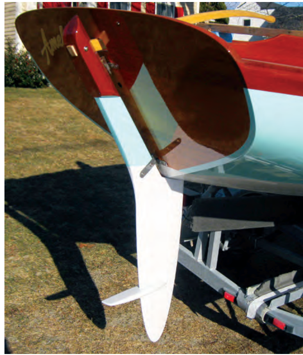
The partially balanced rudder with its rescue step.
