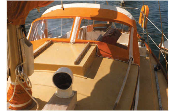
The slats on the companionway hatch cover had holes in them so you could lash the liferaft on top of it.
