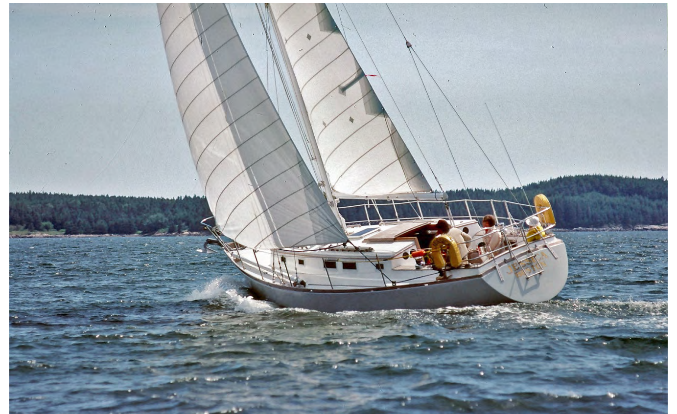
JESSICA was built back in the days of crosscut sails. These narrow panel sails by Hood were the finest you could get.
