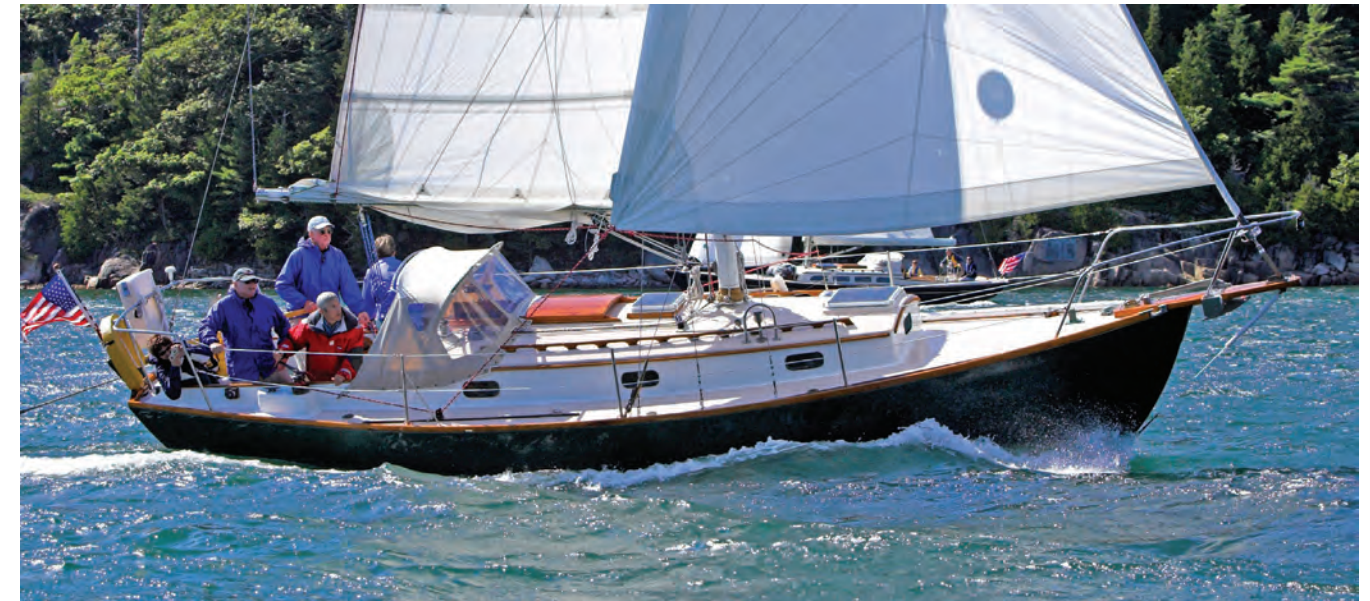
Some of the ANNIES were built with a bowsprit and cutter rig. This moved the sailplan forward. Onne van der Wal photo
