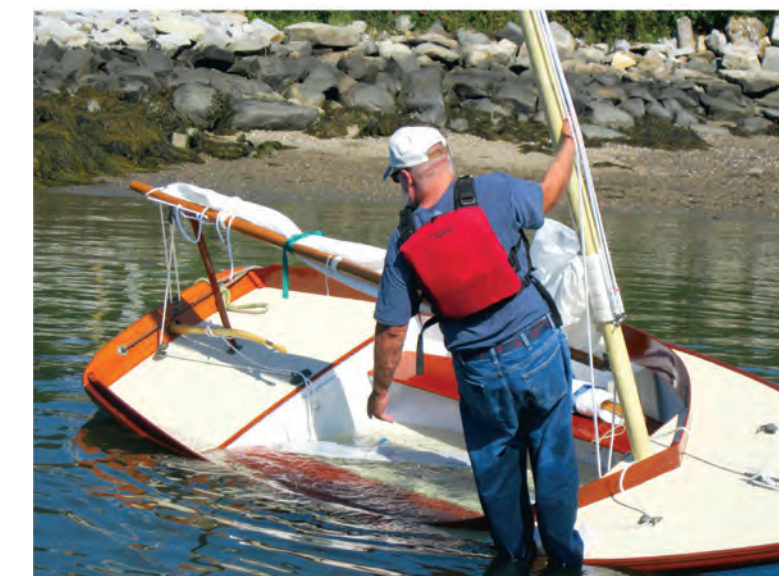
This is how far she can be heeled when fully swamped..
