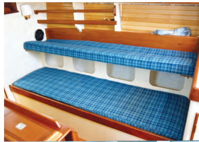
The starboard settee seatback hinged up to form a narrow berth. The leecloth was Velcro'd beneath it.
