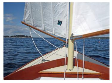
The PAINE 14 carbon fiber mast requires no stays and weighs with its halyards a mere 20 pounds, so it is as easy to deploy as that on a Laser dinghy. Easier, actually, as the sail need not be attached before stepping the mast. We invented a nifty way to attach the sails to the spars very quickly... no tedious fitting of little slides to little tracks, so the boat can be launched and gotten going in a matter of minutes.
