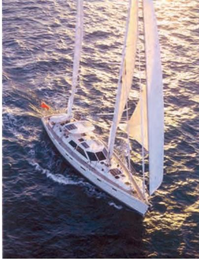
LEONORE was ketch rigged to reduce the size of each sail. Note all the solar panels and the "hard" Bimini.
