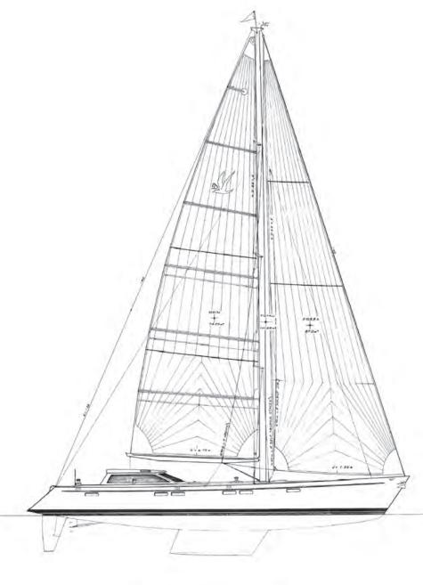
The rig was tall for a light displacement yacht, and situated far forward on the hull. It balanced perfectly. The cutter rig was a bit of an experiment. The foot of the staysail aligned precisely with that of the jib. It worked exceedingly well.
