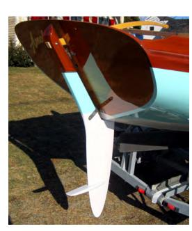
The partially balanced rudder, showing the rescue step.
