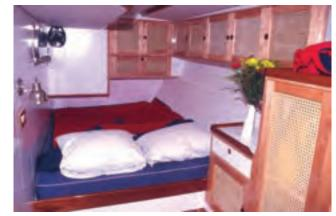
Caned locker fronts were used to eliminate mildew.
