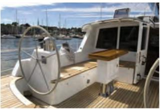
The cockpit was on a single level. The twin wheels were way outboard so you could see past the pilothouse.
