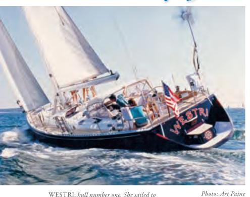
WESTRI, hull number one. She sailed to Antarctica and back. APOGEE 50s were seriously fast with their very long waterlines and light displacement. WESTRI had in-mast furling, which I've never liked. It makes the mast too big.
