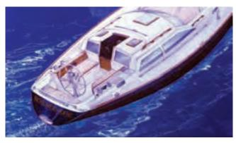
The aft cockpit drawing by Art Paine. It showed the bent side windows, faceted aft face of the pilothouse, teak clad area forward of it—purely for looks—and varnished wood hatches that were always favored by the Hinckley Company. Most important, though, it showed the name of Shep's boat.
