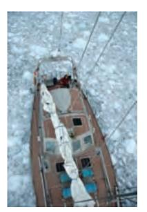
SEAL was designed in anticipation of conditions like this. She is the strongest aluminum hulled yacht our studio ever designed. Her rudder could safely hit an iceberg, which it once did at a speed that would have damaged a conventional fixed rudder beyond any hope of repair.
