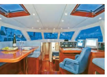
The pilothouse had a dining area to port with the inside steering station to starboard. We always put the steering station on this side because vessels with the right of way, whether under power or sail, come from this direction.
