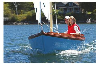
She has nearly identical ergonomics to a H12½—just a tad smaller. You sit on the perfectly slanted wooden seat, lean back and the cockpit coaming cradles your back like a kitchen chair, your hand falls onto the elliptical rounded knob of the tiller, and your feet against the edge of the opposing seat when she heels. The carbon mast is inserted into a fiberglass tube like a Laser dinghy so no stays are required. In anything less than 20 knots of wind, she's considerably faster than a 12½.
