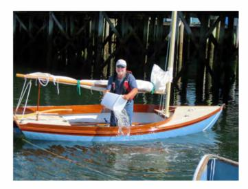
She floats with about ten inches of freeboard when fully swamped. If you swamp an original H 12, the bow tank will keep her afloat for awhile, but floating with the bow pointing straight up, and no place to safely await rescue. Not so the PAINE 14.
