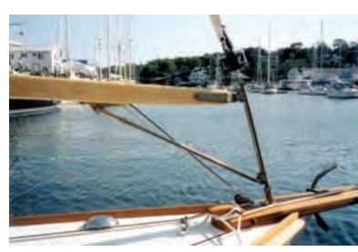
The custom bronze staysail vang enabled the staysail to be roller furled, and kept the boom from "kiting" when off the wind in heavy air.
