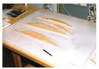
Tracing around the lifts to create the lines drawing.
