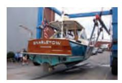
The propeller tunnel shows clearly. You could run aground and wade safely ashore.
