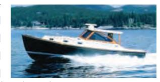
Hull number one, fitted with twin 420 hp Cummins', teak pilothouse and sliding side windows, running at 26 knots. She could go over 30 at wide open throttles.
