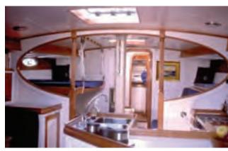
Note the heel-adjustable bunks, held in place by handy billies adjustable from within the berths. These cushions could be lowered down to vertical to be used as seatbacks.
