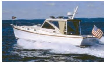
PURITY trimmed level at a speed of 20 knots and didn't throw a lot of spray.
