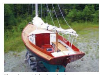
This one has a teak deck and an inboard engine.
