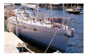
The sharp entry, full length guard rails, and strong anchor roller are obvious as are the ten dorade vents for ventilation.
