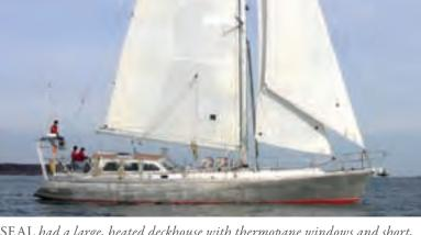
SEAL had a large, heated deckhouse with thermopane windows and short, sheltered cockpit—seldom used in the severe subarctic weather. The deck reels housed lines for mooring to shore, anchors being useless in the conditions often encountered by SEAL's adventure charters. The aluminum was unpainted since scraping against ice was unavoidable.
