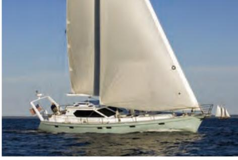
The pilothouse was large, benefiting the interior. The design was all about space and viewing the surroundings, hence the large windows. The arch over the transom was hydraulically operated to double as a gantry to stow the dinghy.
