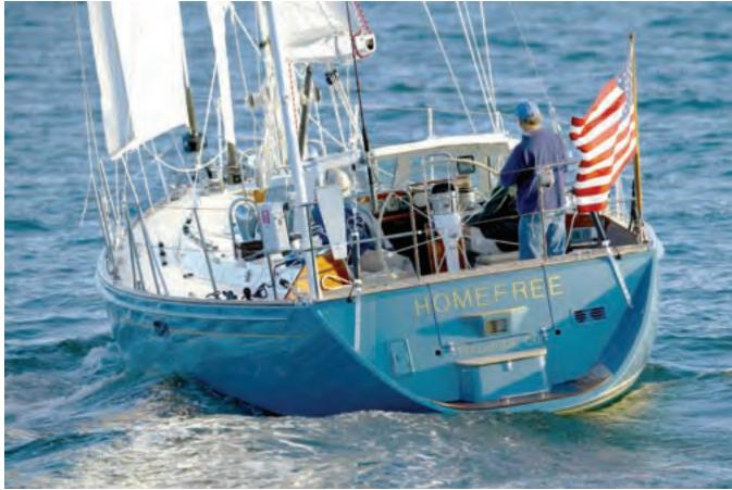
The MORRIS 51 has a molded fiberglass dodger over the companionway. Two people can sit beneath it out of the wind and spray. The varnished spray deflectors continue forward as seatbacks, which adds a warm note of color to the cockpit. HOMEFREE has been sailed around Cape Horn and back.
