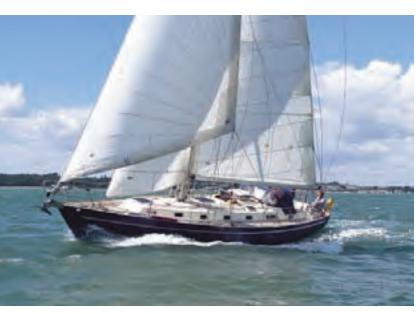
The BOWMAN 42 with her deeper keel and rudder was faster than the 40. With her high-cut yankee and loose-footed staysail she was as efficient as a cutter could be.
