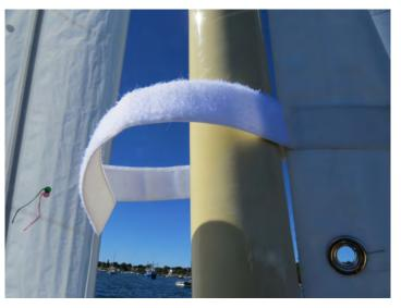
Strap open. The simple Velcro-strap attachments render obsolete tracks and slides, and mast hoops, with all of their expense and tedium, and make getting a small boat rigged and sailing almost instantaneous.
