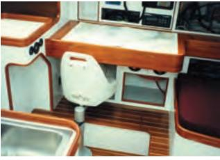
The nav table had a lightweight helm seat that could be rotated into three different positions that all made sense.
