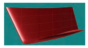
The Scheel Keel had been an idea before its time. It had a voluminous bulb, just as virtually all cruising keels now have, thirty years later. But it also had a small crease that crossed the flow streamlines, adding a bit of drag that seemed unnecessary. And most importantly, the Scheel Keel lacked an endplate.
