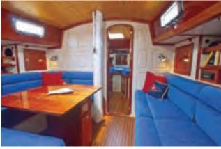
One owner wanted a traditional look, so the plywood structural bulkhead was overlaid to mimic raised panels with rails and stiles.
