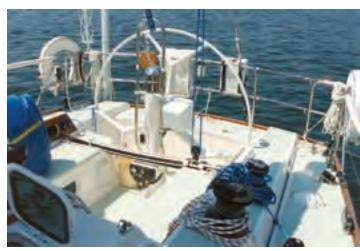
The large carbon fiber wheel got the helmsman outboard for visibility.
