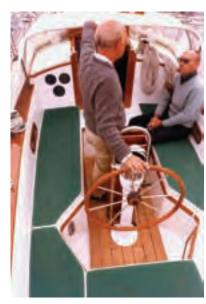
In the early days of fiberglass yachts anything that was different from a wooden yacht was looked at as an innovation. Here it was the nicely tooled notches adjacent the wheel to made it easier to get from forward to aft of the wheel without climbing up on the seats.
