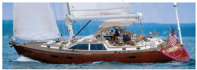
FAR OUT has a tall genoaless rig, teak decks and over-the-top amounts of varnished teak trim which the owner asked me to design personally. I'm especially proud of the pillow shaped name board.
