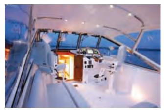
The stainless steel windshield maximized the glass area. Stainless steel is very strong so a little of it goes a long way, structurally.
