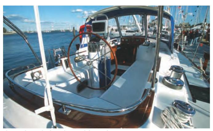
The seats are long enough to sleep on, there are notched coamings for easy entrance, and good sightlines over the low pilothouse. The notches are put directly abreast the wheel—the one place you would not need seatbacks anyway.
