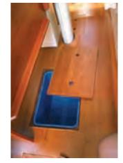
Stowage tubs beneath the sole. You could remove the tubs to check the bilge.
