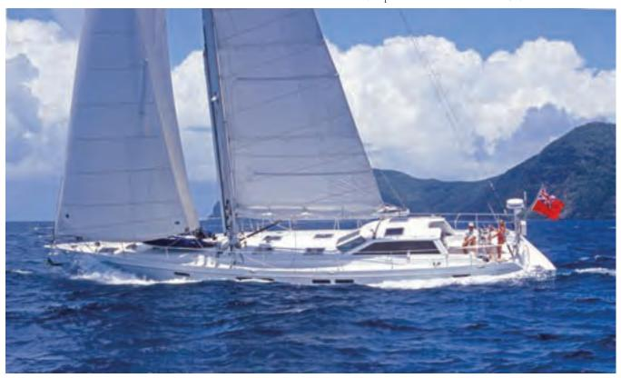
Eric Duttenhofer waves goodbye to Bequia at eleven knots with Laura at the helm. The unusual cutter rig with the low cut yankee and mast well forward worked well. Unlike most cutters, setting the staysail made a perceptible difference in speed.
