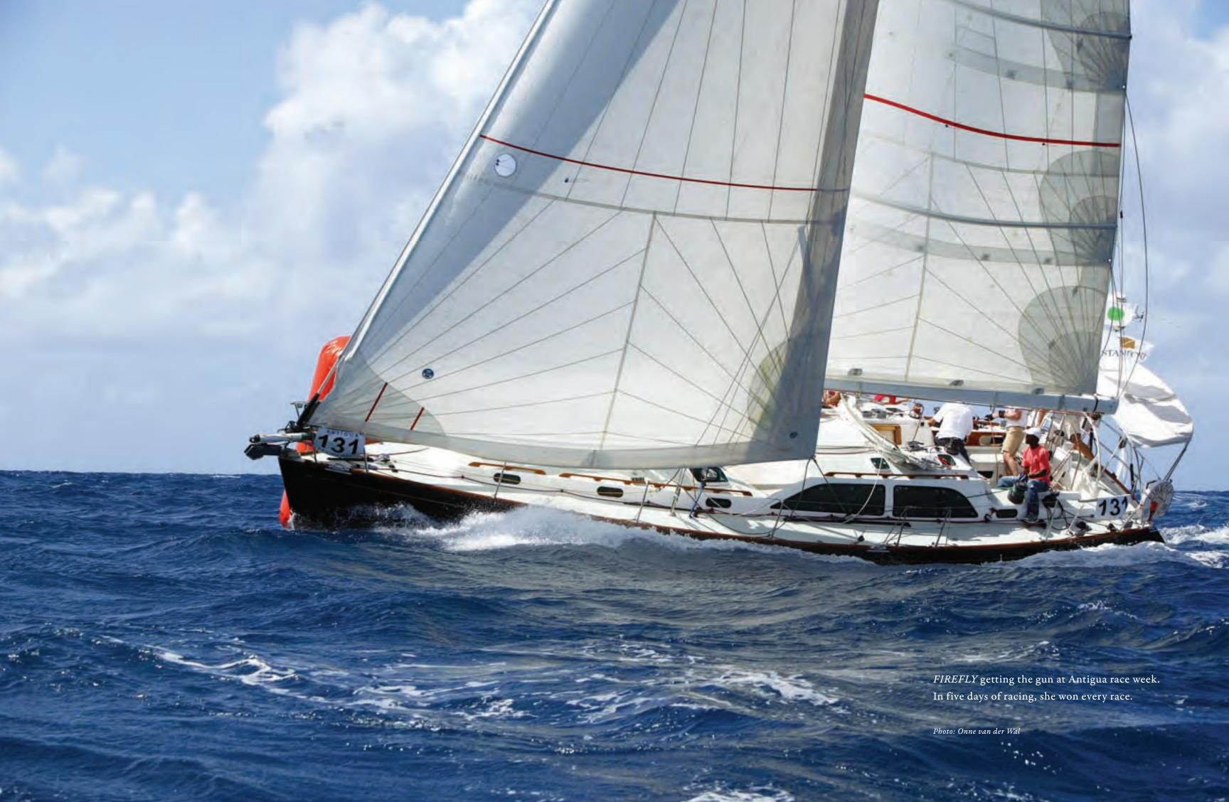
FIREFLY was a scale-down of REINDEER. She had a similar extremely fair hull, the stainless steel and lead bulb keel, the bent windows, and a cockpit with seatbacks forward of the helm. She avoided the extremely lightweight construction that was required for first place grande prix finishes. This flimsy type of yacht has perhaps a three year useful life. FIREFLY was very strongly built, and will still be racing in twenty years' time.
