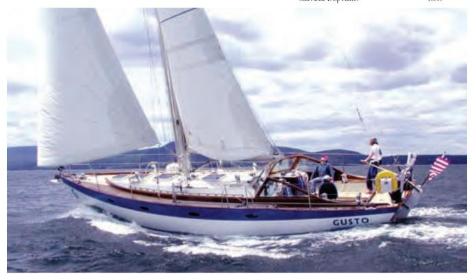
Note the pointed front to the raised deck, the sinuous shape of the upper edge of the windscreen, the elliptical hull windows disguised by the painted wale stripe...yacht design is ART!
